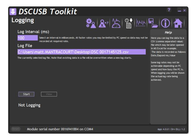
The toolkit allows you to log data to a CSV (Comma Separated Value) file. This file will open in MS Excel when double clicked.
