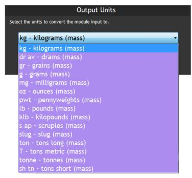
Select the required units, click OK then click the 'Convert' button. The Toolkit will then alter the user calibration to provide the output in the selected engineering units.
