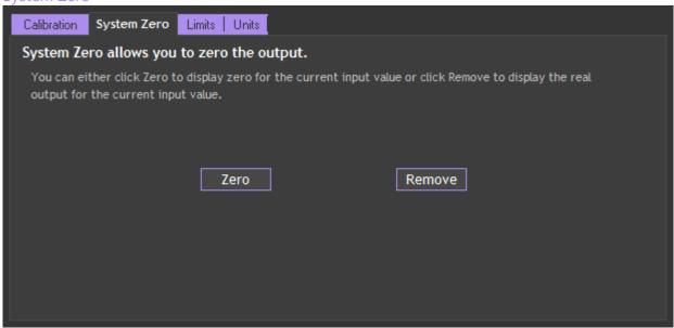
To remove the current weight on all subsequent readings click the '**Zero'** button. Click the '**Remove'** button to return to displaying the actual weight applied. This system zero is stored in the module and remains through power cycling.
