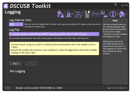
Once the logging starts the actual achieved log rate will be displayed at the bottom of the window. This is useful for diagnostics such as when a heavily burdened PC is slowing the log rate.
